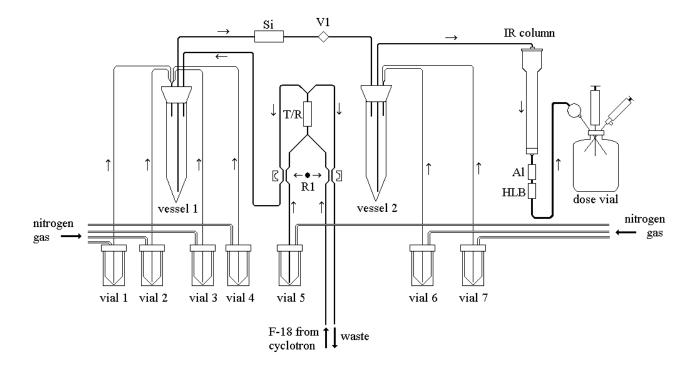
**Figure 1**. Diagram of the CPCU setup for production of *anti*-[<sup>18</sup>F]FACBC. Chemistry occurs in vessels 1 and 2 while reagents are delivered from v-vials 1 through 7 at the appropriate times under positive nitrogen pressure. Arrows indicate direction of flow. Oil heating baths for vessel 1 and vessel 2 are not shown.
