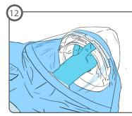
**Slide** the helmet into the hood until it snaps in the center hole. **Snap** helmet into the hood on the left and right side snaps of the face shield.
