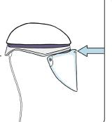
Attach the left and right side lens cuff mounting holes over the left and right side attachment posts of the helmet.
