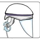
Hold the helmet near the rear headband with one hand, pull down on top of the lens cuff with the other.
