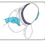
**Place** the chin into the lens cuff while pulling the helmet over and down on the head.
