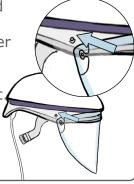
Lift the cuff flappers to rest against the foam pads at the ends of the comfort strip.
