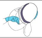
(15) Place the chin into the lens cuff while pulling the helmet over and down on the head.
